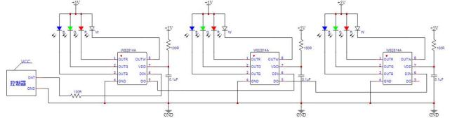
2.12V供电应用参考电路(每通道带3颗LED): 12V power supply application reference circuit (each channel with 3 LED):
