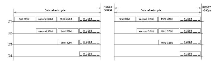
Note: D1 is the data sent by the MCU, and D2, D3, and D4 are the data automatically shaped and forwarded by the cascade circuit.
