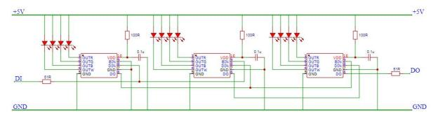
12V power supply application reference circuit (each channel with 3 LEDs):
