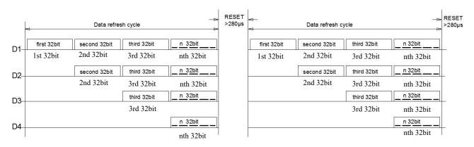
Note: D1 is the data sent by the MCU, and D2, D3, and D4 are the data automatically shaped and forwarded by the cascade circuit.
