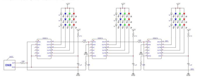
24V供电应用参考电路(每通道带6颗LED): 24V power supply application reference circuit (each channel with 6 LEDs):
