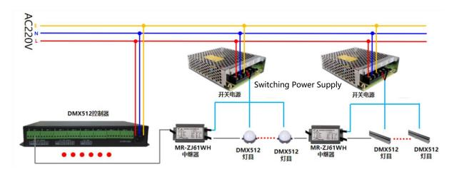
In the use of MR-ZJ61WH signal amplifier, the input and output are fully isolated by the signal port, so the wiring must not connect the ground (GND1) of the input to the ground (GND2) of the output.
