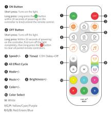
Support one-to-many control, one remote control can control multiple controllers.
