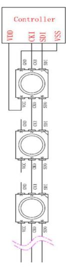
In the practical application circuit, the signal input and output pins of the IC signal input and output pins should be connected
