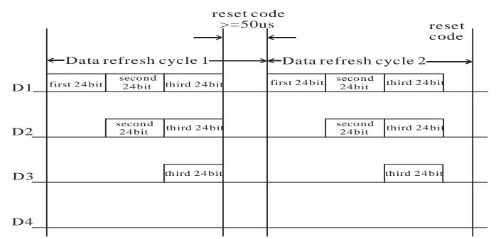
Note: the D1 sends data for MCU, D2, D3, D4 for data forwarding automatic shaping cascade circuit.
