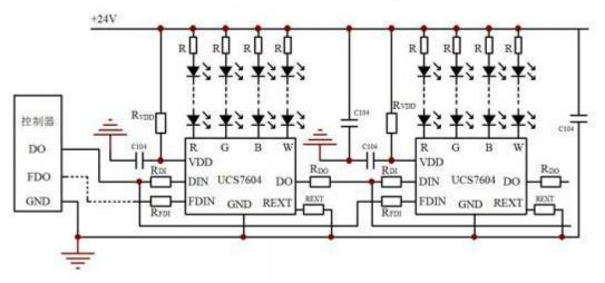
Note 1: In the application, the connection between the controller FDO and UCS 7604 is not connected, so the first point does not have a complete breakpoint transmission function.
