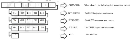
RI [bit15~bit11]:Set R channel constant-current value, Ir=10+RI[4:0]mA, namely minimum 10+0=10mA, maxium 10+31=41mA
