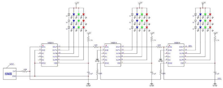
2. Supply voltage=24V(Each channel drives 6LEDs)
